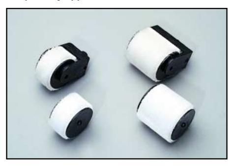
Semco® roller nozzles are designed to apply adhesives and sealants evenly over a wide area of substrate. They are ideal for the application of faying surface sealants. The ¹/₄ NPT male threaded end can be used with any of the Semco® line of disposable cartridges and Semkit® packages (i.e. 1, 2.5, 3.5, 6, 8, 12, 20, 32 oz. and ¹/₁₀ gallon sizes).
