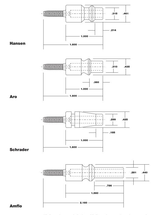
All dimensions are in inches. All dimensions are for reference only. Modified thread fits P/N 220895 (bulk gun hose).
