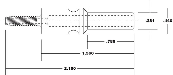
**All dimensions are in inches. All dimensions are for reference only. Modified thread fits P/N 220895 (bulk gun hose).**
