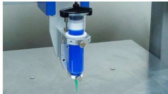
6. Install syringe and lightly tighten thumb screws.
